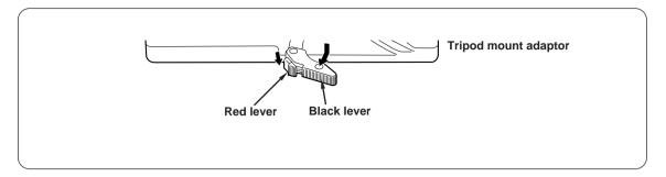
Move the black lever in the direction indicated by the arrow while holding down the red lever, and disengage the unit by sliding it toward you.
